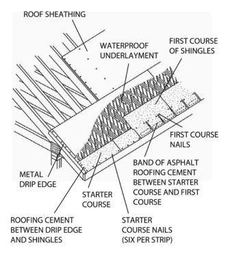
The roof sheathing (typically plywood panels) should be at least 15/32 inch thick and securely attached to the roof trusses. (Nails in older wood roof sheathing often are farther apart than recommended, especially in areas subject to high winds). Your roof designer or roofing contractor should
